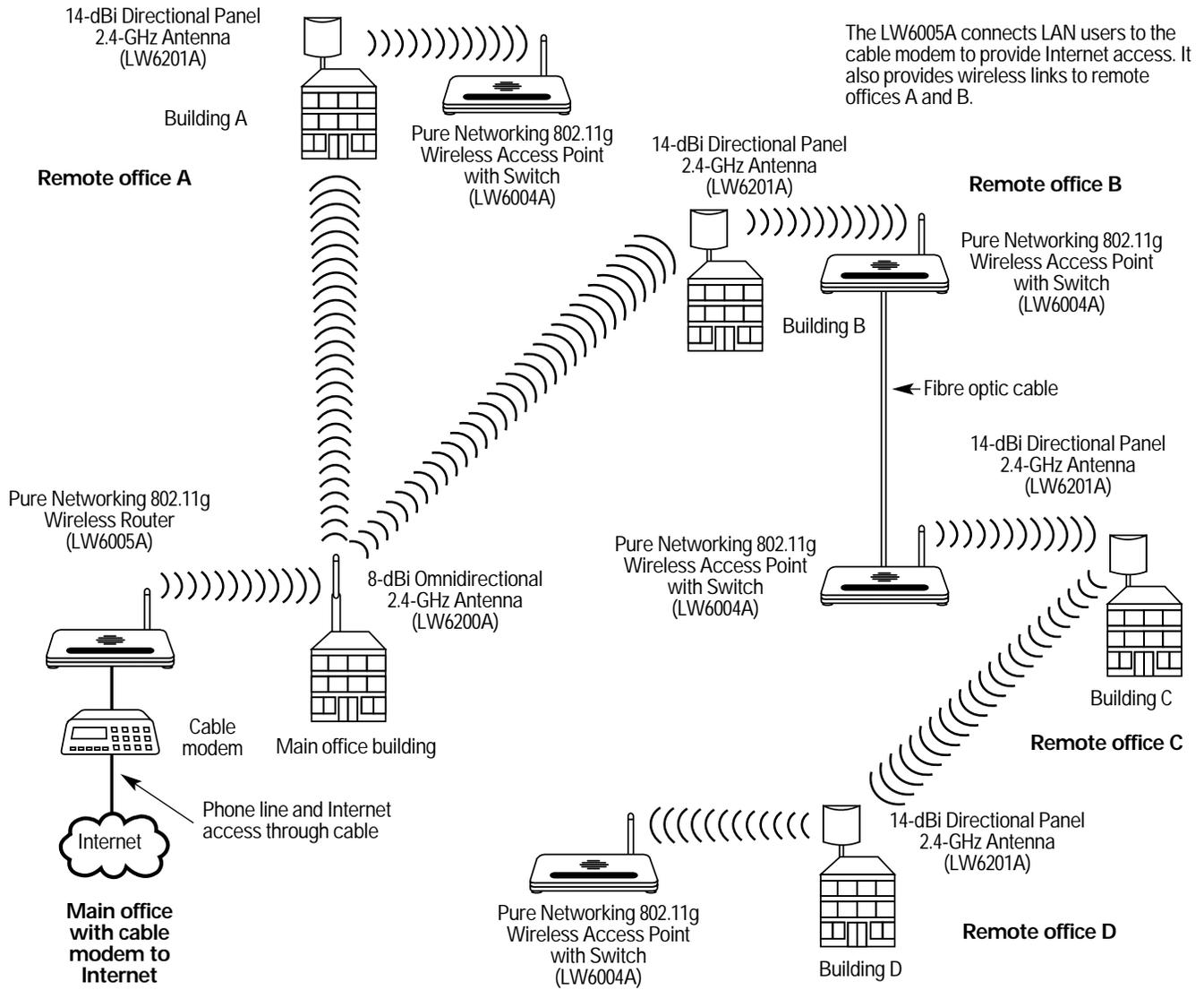
Offices C and D do not have a clear line-of-sight to the main office, so office C was connected to B over fiber optic cable. A wireless link was then set up between C and D.
