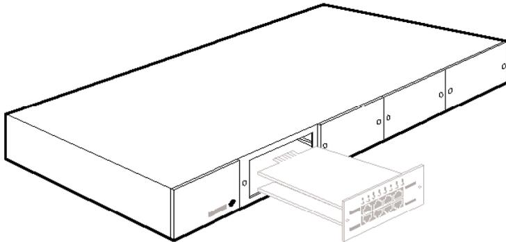
*Each chassis slot functions as a MAU, an RI/RO unit, or a Repeater—just add the appropriate module!*
