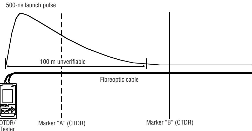
*...but with the Equalizer, the problem of launch pulses masking the initial length of fibre is greatly reduced, and you can get accurate measurements—right from the start.*
