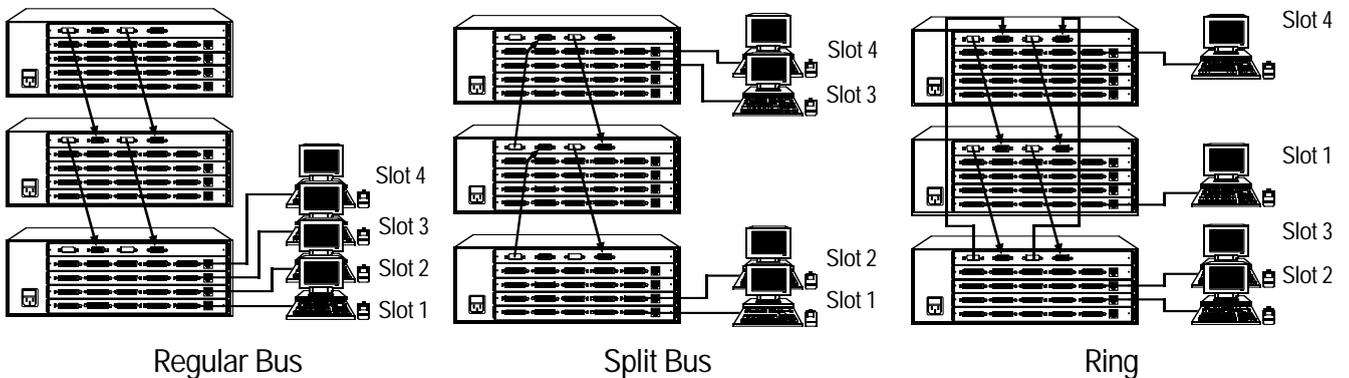
\*Keep in mind that only one user at a time can use the bus that interconnects daisychained Affinity units, especially when you implement a ring topology. For example, when your Affinity units are interconnected in a ring, if any user on slot 1 selects a CPU attached to an Affinity unit other than his own, no other slot 1 user can select any CPUs.
