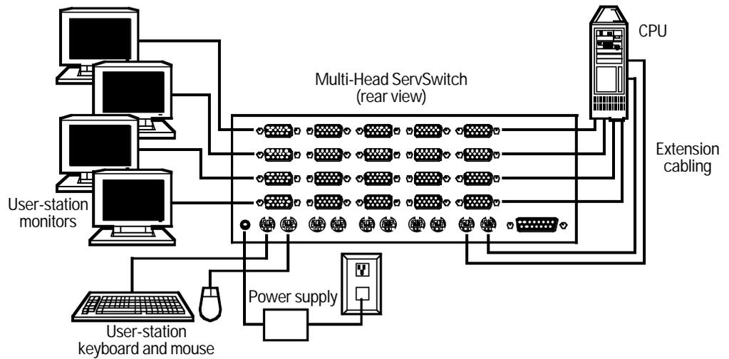
NOTE: For clarity, only one CPU is shown. Also, though separate extension cables are shown here, we recommend that you use our special Premium KVM CPU Cable (EHN408) to connect your CPU's first video port and its keyboard and mouse ports to the Switch. This cable has a central video strand with keyboard and mouse strands bonded to either side.
