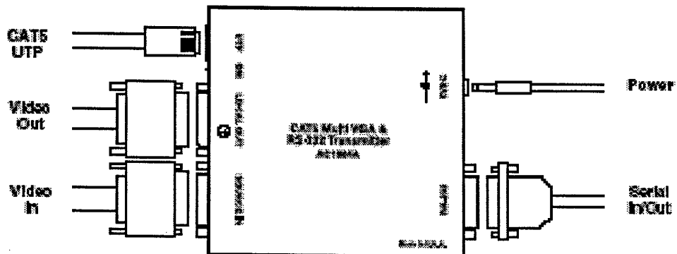
Figure 3-3. Transmitter connections on the AC1004AR2.
