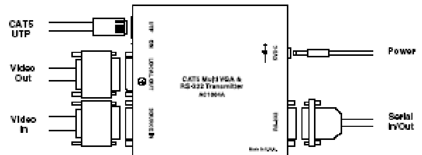
Figure 3-3. Transmitter connections on the AC1004A.
