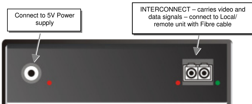
DVI-D KVM Extender KVM-Extender Type ACS1009A-xx Local/ Remote Unit
