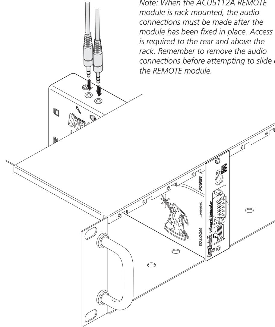
Note: When the ACU5112A REMOTE module is rack mounted, the audio connections must be made after the module has been fixed in place. Access is required to the rear and above the rack. Remember to remove the audio connections before attempting to slide out the REMOTE module.
