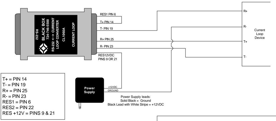
CL1060A can be ordered with a male or female DB25 Current Loop connector. The RS-232 connector is only DB25 female.
