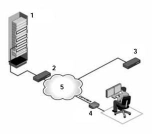
Figure 2-1. DTX Extender System - Desktop Mode
