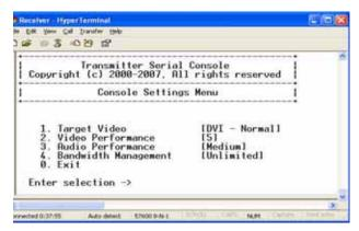
Figure 4-37. Transmitter Console Settings Menu
