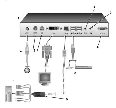
Figure 3-3. DTX5000-R User Station and DTX5000-T Transmitter Installation
