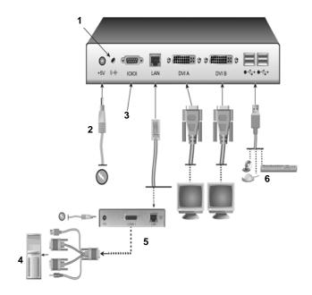
Figure 3-7. DTX5002-R User station and DTX5002-T transmitter Installation
