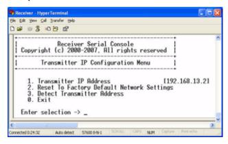
Figure 4-14. Transmitter Configuration Menu on the DTX User station
