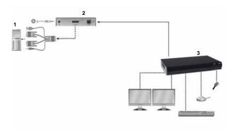
Figure 3-5. Point-to-Point Installation (DTX5002-R and DTX5002-T)
