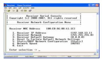
Figure 4-17. Receiver Network Configuration Menu (Extender and Matrix Mode)
