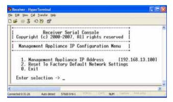
Figure 4-19. DTX5000-CTL Management Appliance IP Configuration Menu
