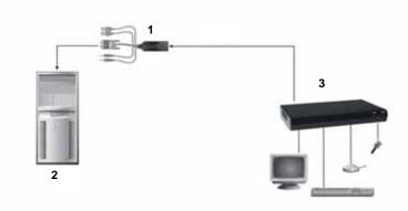
Figure 3-1. Point-to-Point Installation (DTX5000-R User Station)
