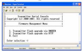
Figure 4-25. Transmitter Firmware Management Menu
