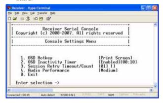
Figure 4-35. Receiver Console Settings Menu
