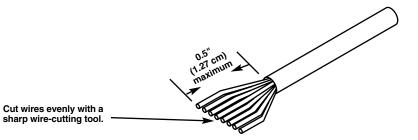
Figure 1. Making sure the wires are cut evenly.
