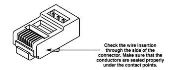
Figure 3. Checking the insertion.
