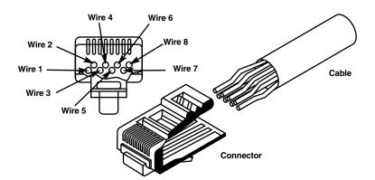
Figure 2. Inserting the cable wires into the connector.
