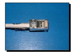
6. Hold Conductors in proper order. Insert into Plug Body. All conductors should be bottomed in the plug housing . Make sure shield and or drain wire is positioned to contact the ground fingers in the bottom of the plug opening. Terminate in proper
