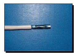
Pull back foil shield, wrap drain wire around foil and cable jacket. Optionally, remove foil flush with jacket and wrap drain around cable jacket.
