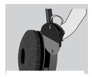
Figure 3-5. Removing the Chamber from the Headset.
