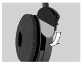
Figure 3-7. Putting the Battery Chamber Back into the Headset.
