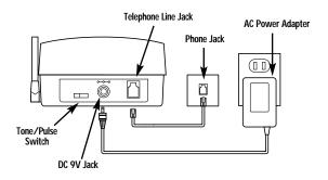
Figure 2-2. Connecting the power adapter to the jack on the base unit.
