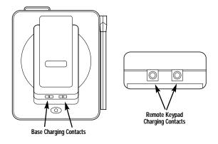
Figure 2-7. Checking the battery connections.
