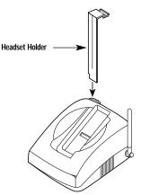
Figure 2-1. Connecting the headset holder to the base unit.
