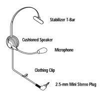
Figure 3-1. Parts of the Headset.
