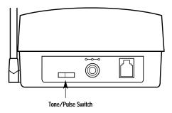
Figure 3-3. Setting the tone/pulse switch.
