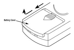
Figure 2-3. Removing the cover.
