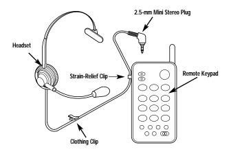
Figure 2-5. Installing the headset.
