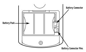
Figure 2-4. Connecting the battery pack.
