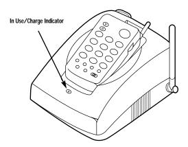
Figure 2-6. Putting the keypad in the base.
