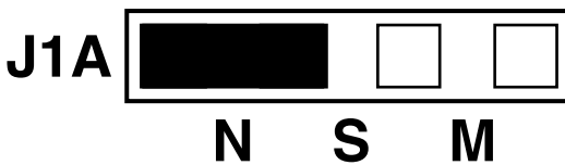
Figure 3-3. Header J1A, Normal IRQ Mode.
