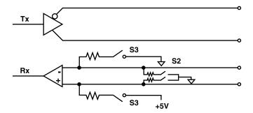
Figure 3. Line bias. S2 shows the line termination when "Term" is selected. S3 shows line bias when "Bias" is selected.
