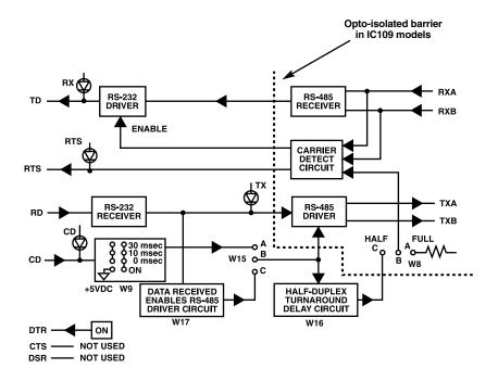
Figure 4. Simplified functional block diagram (DTE operation).
