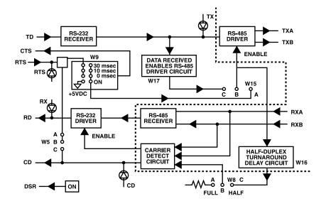
Figure 2. Simplified functional block diagram (DCE operation).
