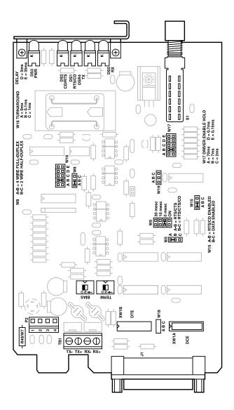
Figure 1. The printed circuit board's layout.
