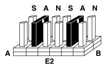
Figure 3-4. Jumper block E2.
