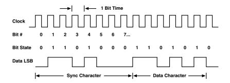
Figure D-2. Synchronous communication.
