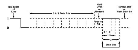
Figure D-1. Asynchronous communication.
