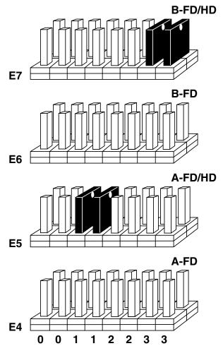
Figure 3-3. Jumper blocks E4 through E7.
