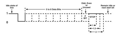
Figure B-1. Asynchronous Communications Bit Diagram.
