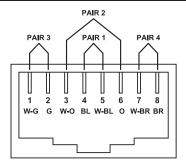
Figure 5-2. T568A wiring.
