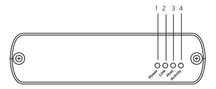
Figure 2-1. Front panel of the local unit.
