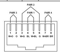
Figure 5-3. T568B wiring.
