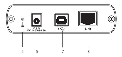
Figure 2-2. Back panel of the local unit.
