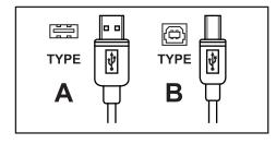
Figure 4-1. USB Type A and Type B cable connectors.
