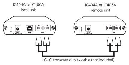
Maximum 500 m multimode fiber for IC404A; maximum 10 km single-mode fiber for IC406A Trademarks Used in this Manual
