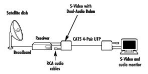
Figure 3-1. Satellite S-Video and audio typical application.
