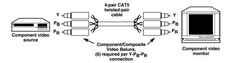
Figure 3-2. Component video connection.
