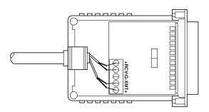
**10.** Bend the top half of the case as necessary to place it over the strain-relief assembly. Do not snap the case together yet.
