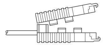
11. Insert one captive screw through a saddle washer, then insert the captive screw with the washer on it through the hole in the DB25 end of the case. Snap that side of the case closed. Repeat the process for the other side. Cable installation is complete.
