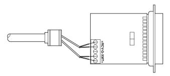
**9.** Insert the strain-relief assembly with the wire going through it into the slot in the bottom half of the modem case and set it into the recess in the case.
