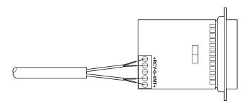
**8.** Place the two halves of the strain-relief assembly on either side of the twisted-pair wire and press together very lightly. Slide the assembly so that it is about two inches (5.1 cm) from the terminal posts and press together firmly.
