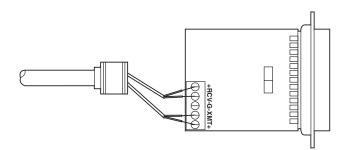
**9.** Insert the strain-relief assembly with the wire going through it into the slot in the bottom half of the modem case and set it into the recess in the case.
