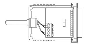
**10.** Bend the top half of the case as necessary to place it over the strain-relief assembly. Do not snap the case together yet.
