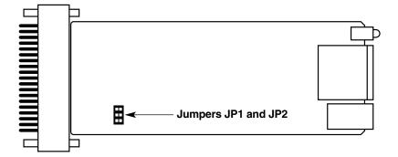
Figure 3-12. JP1 and JP2 (on the top of the IC701A's PC board), as seen when the V.35 connector shroud is removed.
