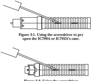
Figure 3-2. Using the screwdriver to pry open the IC701A's case.
