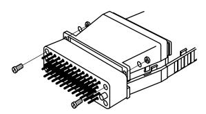
Figure 3-11. Removing the bolts.
