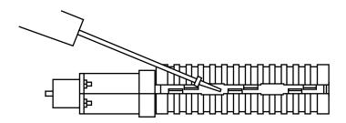
Figure 3-3. Using the screwdriver to completely open the IC700A or IC702A's case.
