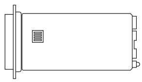
Figure 3-14. Switch S1 (located on the bottom of the IC702A's PC board).
