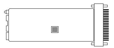
Figure 3-9. Switch S1 (located on the bottom of the IC701A's PC board).
