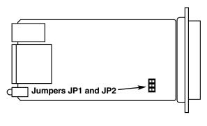
Figure 3-16. (JP1 and JP2 on the top of the IC702A's PC board).
