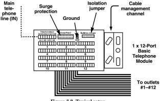
Figure 3-2. Typical setup.
