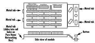
Figure 2-1. 1 x 12-Port Basic Telephone Module.
