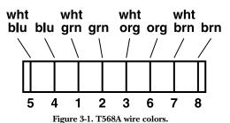
4. To terminate the connection, place each wire into the insulation displacement contacts (IDC) by matching the wire color with the applicable colors on the terminal block (568A).
