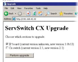
8 Select which portion of the ServSwitch CX with IP that you wish to upgrade. Tick both options to upgrade the complete unit. When ready, click the *Perform upgrade* button.
