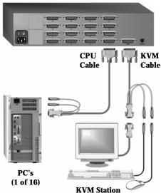
Figure 2. Single Unit configuration
