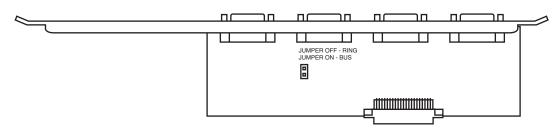
Figure 3. The RING/BUS jumper.
