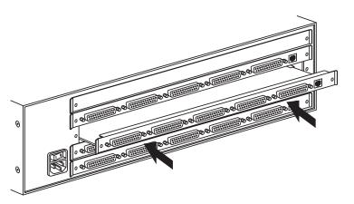
Figure 1. Installing a Port Card.
