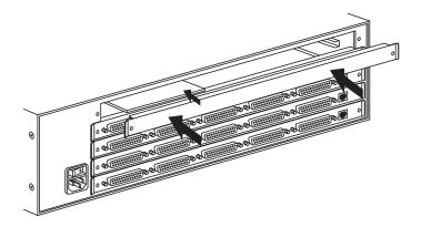
Figure 2. Installing a Terminator Card.
