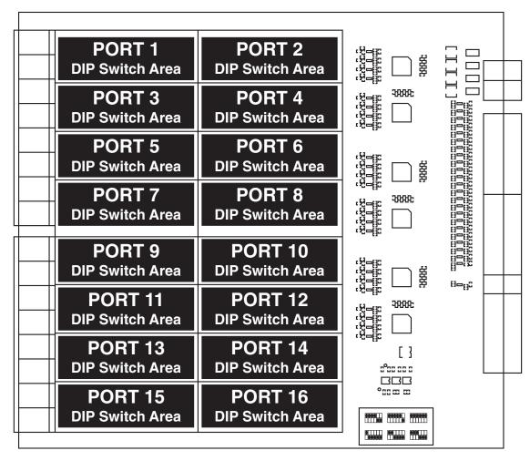
Figure 1. The DIP-switch areas on the Transmit Module's circuit board.
