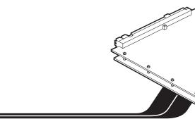
Transmit Modules (product code KV1701C) and their companion Receive Modules (KV1702C) are the components of the ServSwitch Multi Hub (KV170RA) that handle its communication with other ServSwitch Multi units. Here's how to configure and install your Transmit Module:
