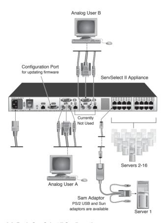
Figure 3-2. Basic ServSelect II Configuration
