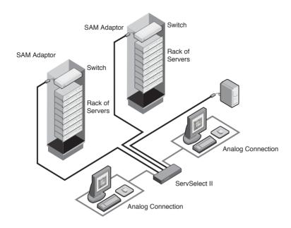
Figure 2-2. Example ServSelect II Configuration
