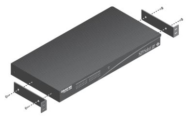
Figure 3-1. ServSelect II Horizontal Installation
