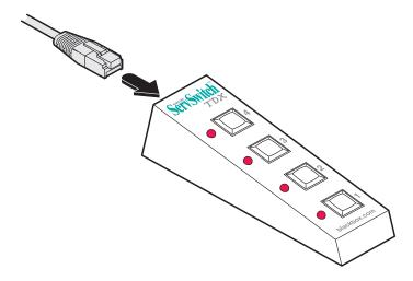
2 Connect the other end of the cable to the **OPTIONS** port on the rear panel of the unit.
