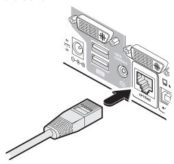
2 Connect the other end of the cable to a vacant serial port on the computer.
