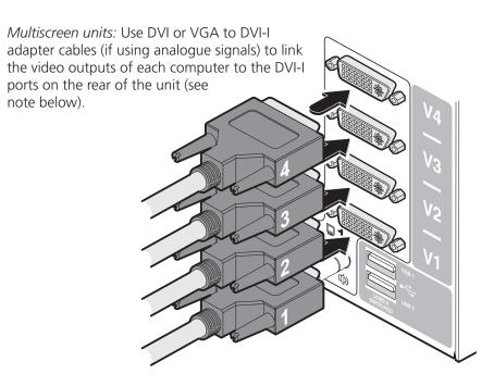
Note: On the rear panel of the unit, connectors belonging to the same channel are stacked vertically. The connectors at each horizontal level (V1 to V4) will be switched through to the user console DVI-I connector which is at the same level:
