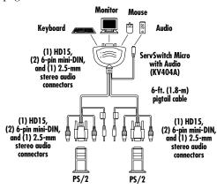
Figure 3-1. The ServSwitch Micro's cable connections.
