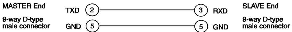
The pinout for a “daisy chain” RS232 cable for more than 2 units is shown below:
