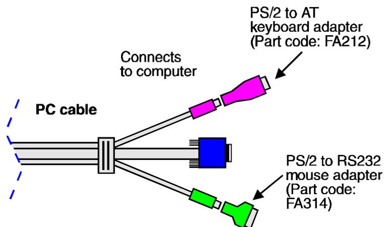
**Cables for connection to Sun computers with 8-pin keyboard/mouse connectors:**
