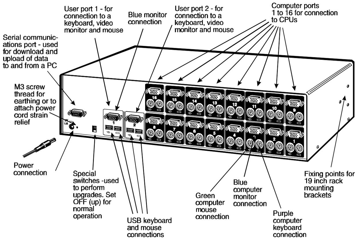
Fig. 2c – KV6616FA ServSwitch Duo USB viewed from the rear
