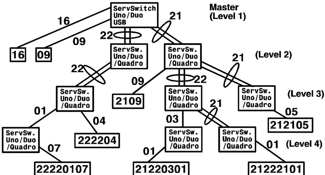
Fig. 6 - Creating menu entries for computers that are connected to cascaded ServSwitches
