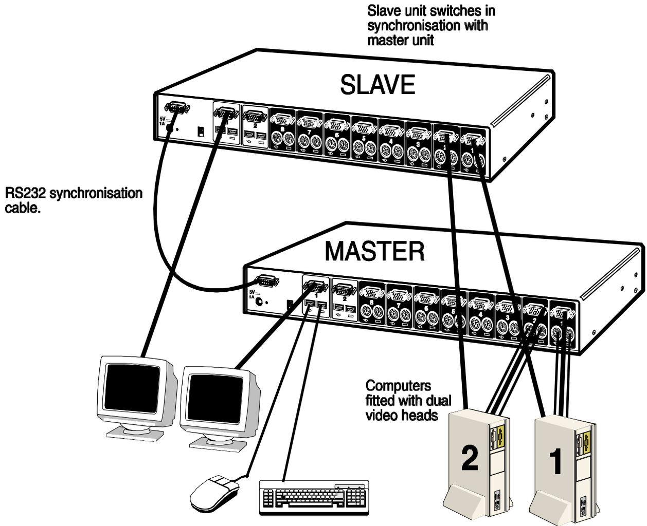
Synchronised ServSwitches used for a dual head video switching application
