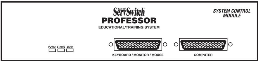
Figure 2-1. The front panel of a ServSwitch Professor.
