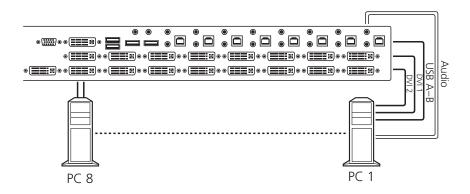
Figure 3-2. Connecting the computer.
