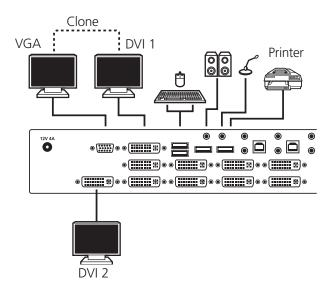
Figure 3-1. Connecting the console.
