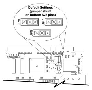
Figure 2.4 Factory Configured Jumpers
