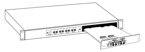
Figure 2.5 Installing a Bridge Module in a Modular Concentrator/2
