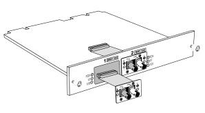
Figure 2.2 Installing a 100-Mbps Module
