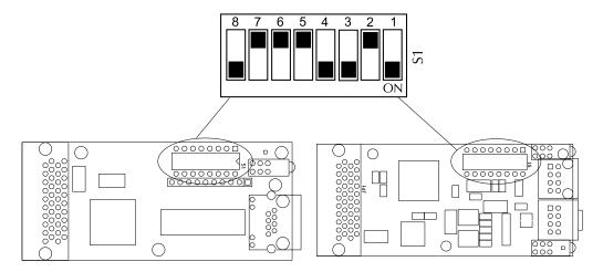
Figure 2.1 8-Position Switch for Configuring Twisted Pair (l.) and Fiber (r.) 100-Mbps Modules
