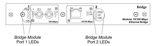
Figure 2.6 Bridge Module LEDs
