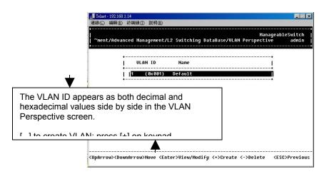
Create VLAN Step 2: Press [+] on keypad to enter New VLAN Settings. Enter new VLAN ID and VLAN name.
