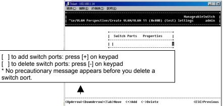
Step 4: Move to highlight a suitable option from **Port Options** and press <Enter>, e.g. Untagged Ports.
