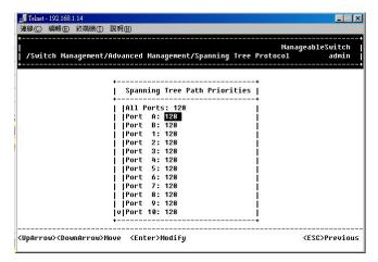
Step 2: Move to highlight **All Ports** or each port individually, and press <Enter>. For new priority value, type a decimal number from 0-255, and press <Enter>. A low value gives the port a greater likelihood of becoming a Root port.
