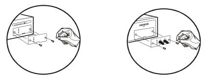
Figure 1: Removal of module cover plate One port fiber module being installed
