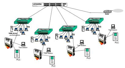
LBH100A-H Converter Switches provided a secure economical solution for expanding Industrial network
