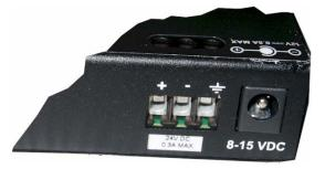
is located on the left side of the unit and is equipped with three (3) screw-down lead posts. The power terminals are identified as positive (+) and negative (-), and they are floating inside the unit so that either of the terminal may be grounded by the user if desired. The chassis is "earth" or ground (GND).
