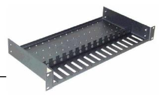
mounted with the DC power jack in the back, with the fiber and the RJ-45 connectors in the front. Any mix of the Media Converter Switches and/or Media Converters may be placed on a tray, up to a maximum of 16 units. (The mounting spaces of the LE1505-RACK are specific to the products and will not permit other models to be properly mounted).
