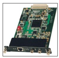
Figure 1 - CityLIGHT 10/100 Ethernet Switch Card
