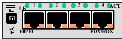
Figure 4.3 : Up-link push-button on RJ-45 4-port
