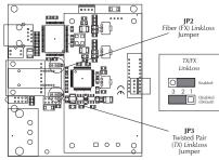
In order to enable TX and/or FX LinkLoss, remove the cover from the Compact Media Converter and place the jumpers accordingly. To do this:
