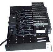
(PoE) Switch, each with their power input plugged into the built-in common AC power supply in the rear area of the tray. (PS units that come with the MC's are not used)..
