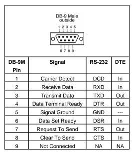
Figure 21. RS-232 Connections in a DB-9 Connector
