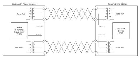
Figure 23. Power over Ethernet Alternative A
