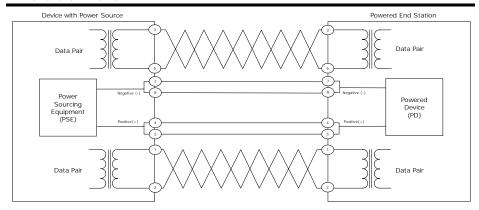
Figure 24. Power over Ethernet Alternative B
