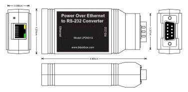
Figure 19. Dimensional Diagram of the LPD401A
