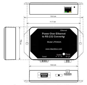
Figure 20. Dimensional Diagram of the LPD402A
