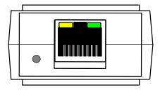
Figure 4. LED Indicators on the LPD401A
