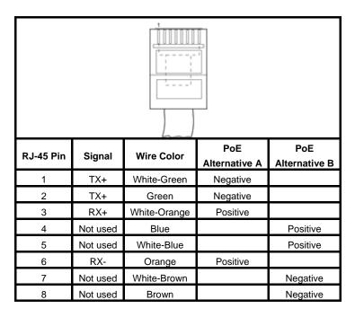
Figure 22. Pin-out for an Ethernet Cable showing PoE
