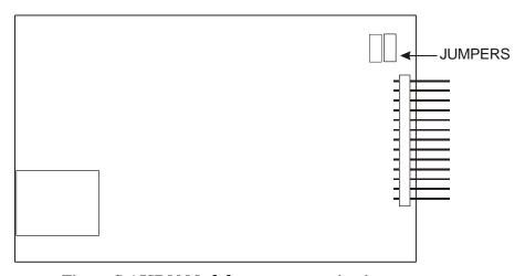
Figure C-4 ISDN Module processor setting jumpers
