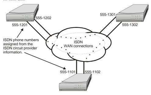
Figure 2 - 5 Basic ISDN Configuration
