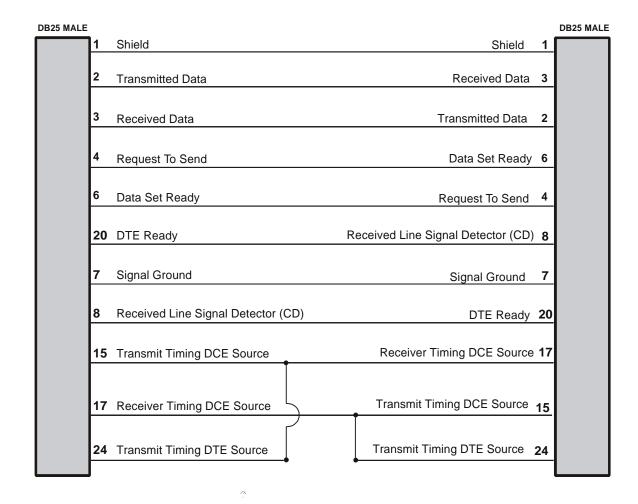
Figure D-9 RS232 Null-Modem Cable
