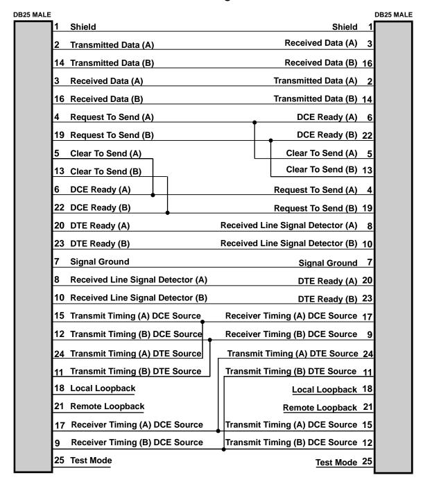
Figure D-11 RS530 Null-Modem Cable
