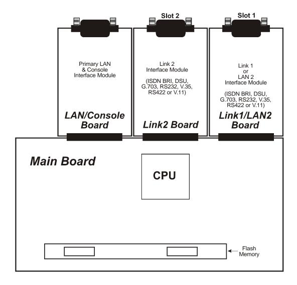
Figure C-1 Top Internal View of the Ethernet Bridge/Router
