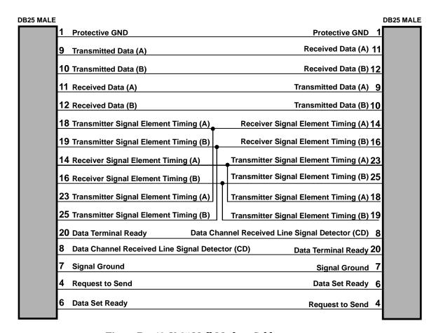
Figure D – 10 V-35 Null-Modem Cable
