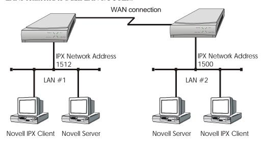
Figure 2 - 3 IPX Routed Local Area Networks (Servers on both sides)
