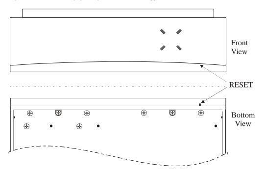
Figure 1-1 Location of the Reset Hole on Router
