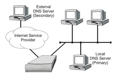
Figure 2-10 Local + External DNS Server Configuration
