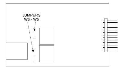
Figure C-5 ISDN S/T Module Termination setting jumpers
