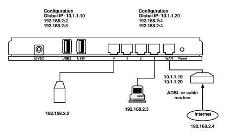
Figure 5-20. Using a virtual server.
