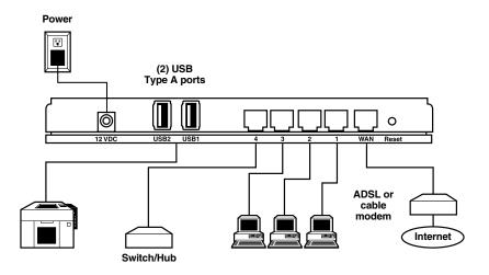
Figure 3-1. Typical LAN setup.
