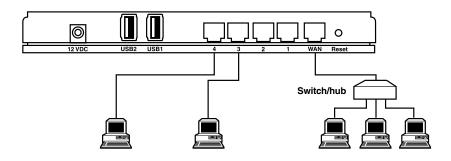
Figure 5-9. Bridge mode configuration.
