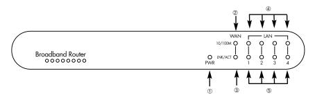
Figure 2-2. Front-panel LEDs.
