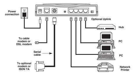
Figure 2-1. Cabling the Router.
